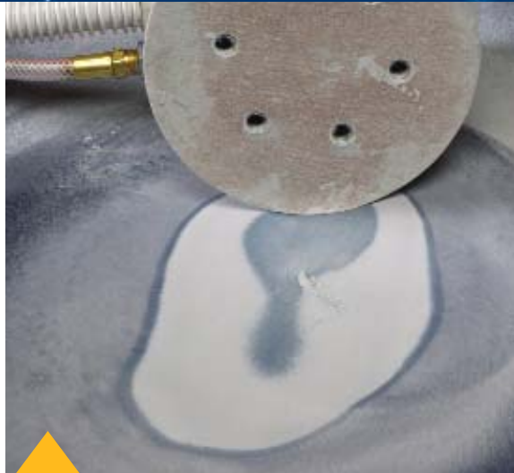
After 3 minutes, a conventional vacuum assist disc is clogged and can create shop contaminants.
